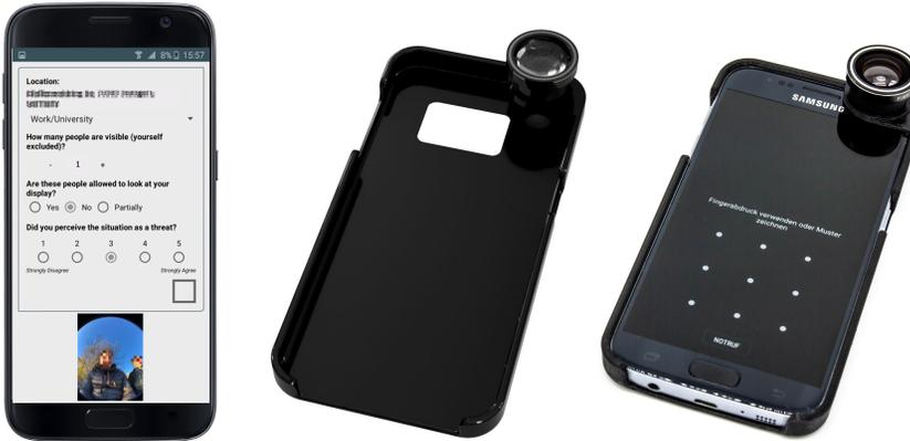
Fig. 2. The rating application (left) and the smartphone enclosure including, fish-eye lens (center: rendered design, right: prototype).
