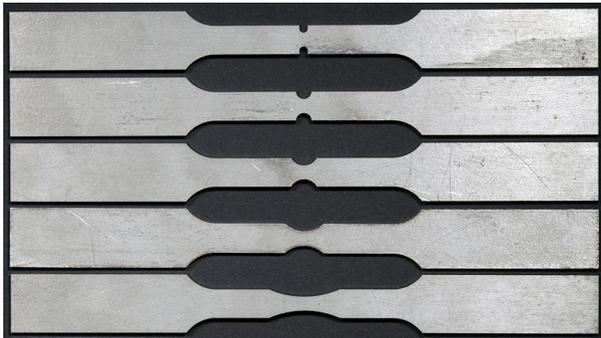
**Figure 4.9:** Tension specimens, series with different notch radius 1.25, 2.5, 5.0, 10.0, 30.0 mm, Inox 304L
