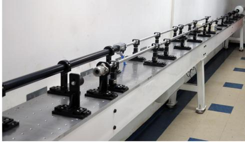
**Figure 4.6:** In situ experimental setup of Split-Hopkinson-Bar at GM-SIE lab, University of São Paulo (USP), Brazil; front: pressure bar with gas gun
