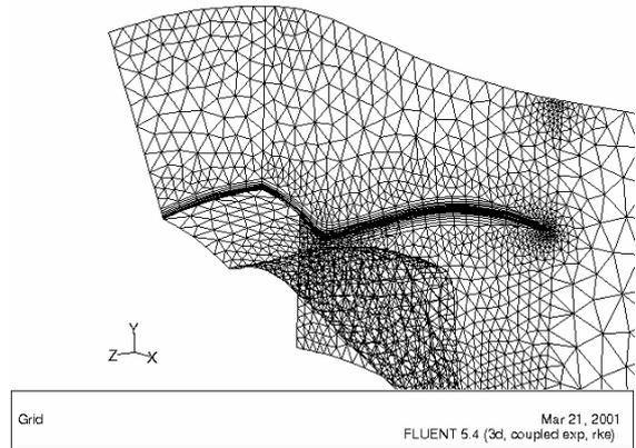
**Fig. 9** Hybrid mesh for BR715 inverse scarfed research mixer
