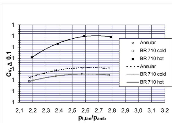
Fig. 3 BR710 16 lobe mixer thrust coefficient
