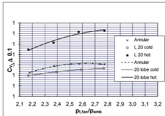
Fig. 5 BR710 20 lobe mixer thrust coefficient
