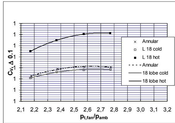
Fig. 4 BR710 18 lobe mixer thrust coefficient
