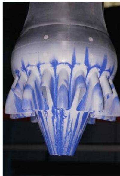
**Fig. 10** Flow Visualization on inverse scarfed mixer
