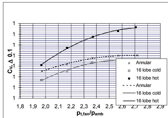
Fig. 6 Tay 611 new 16 lobe mixer thrust coefficient
