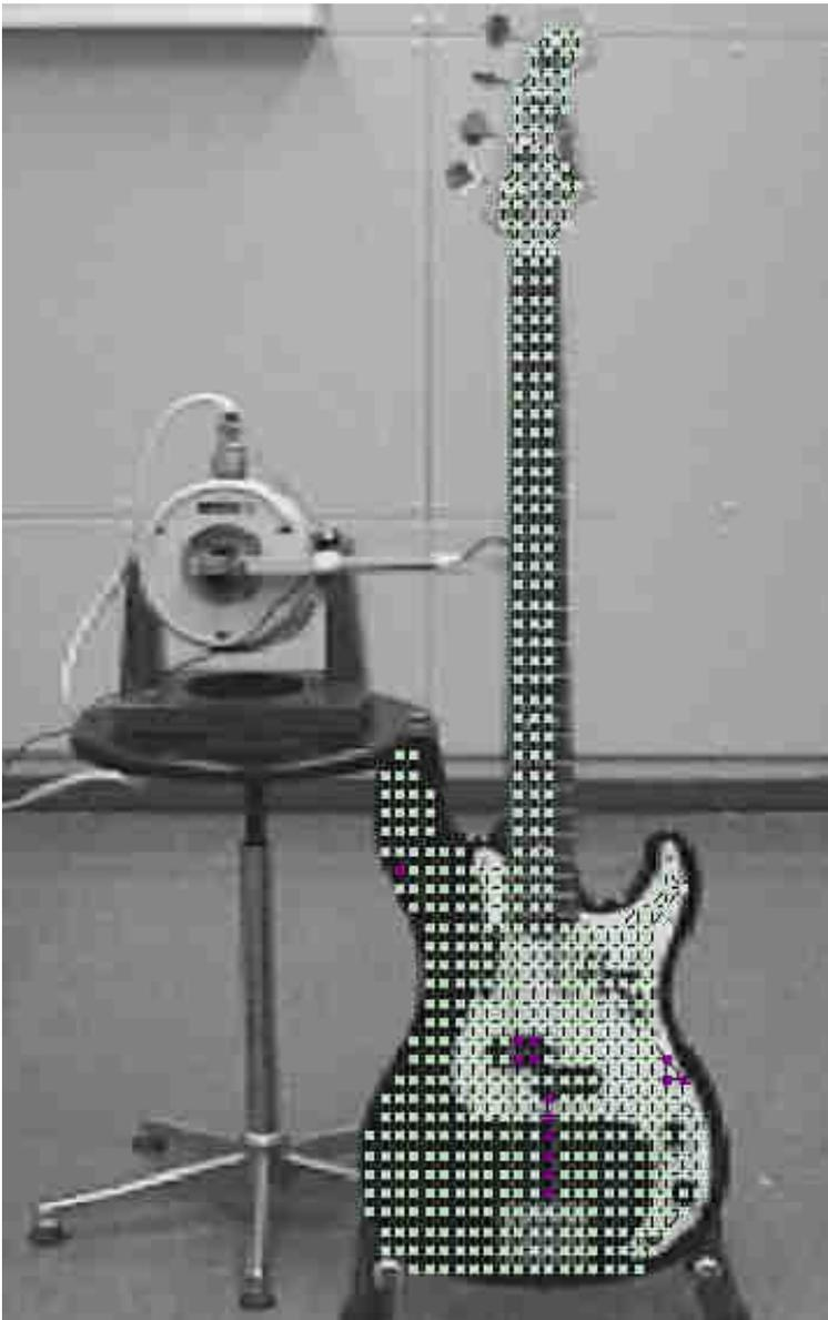
*Fig. 9. Action Bass No. 1 including measuring points during the in-stand determination of the operating deflection shapes by means of the Scanning Vibrometer.*
