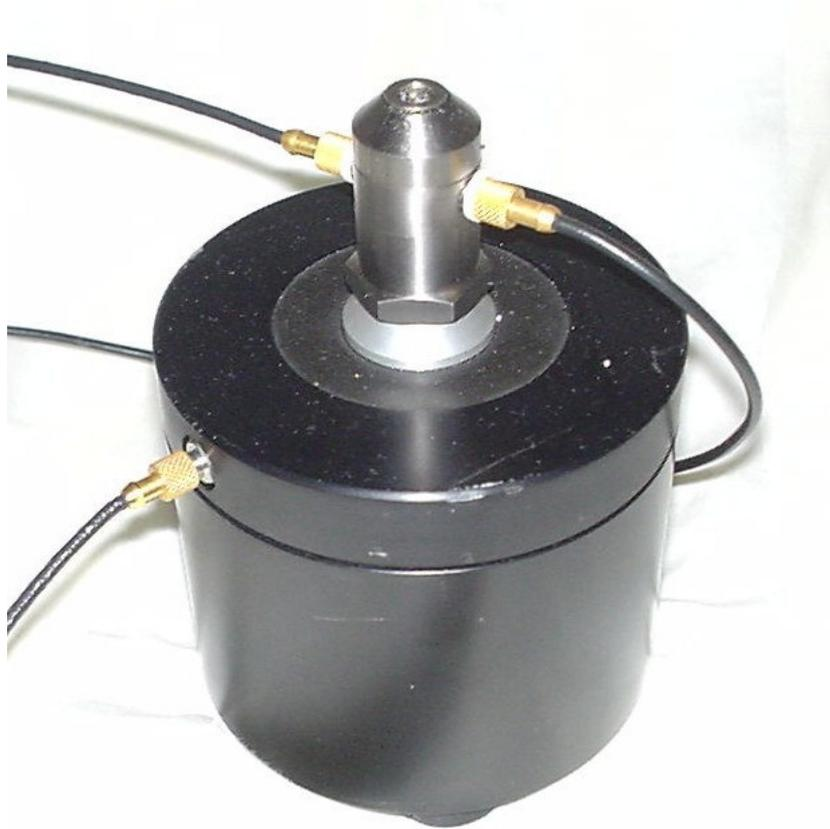
Fig. 21. Impedance head and mini-shaker as used for the conductance measurements.
