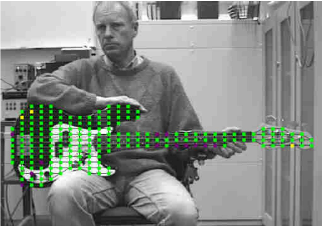
*Fig. 6. Action Bass No. 1 including measuring grid during the in-situ determination of the operating deflection shapes by means of the Scanning Vibrometer.*
