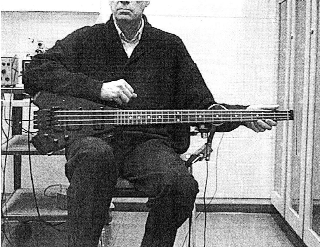
*Fig. 28. Riverhead Bass No. 5 during the experimental determination of the operating deflection shapes by means of the Scanning Vibrometer.*
