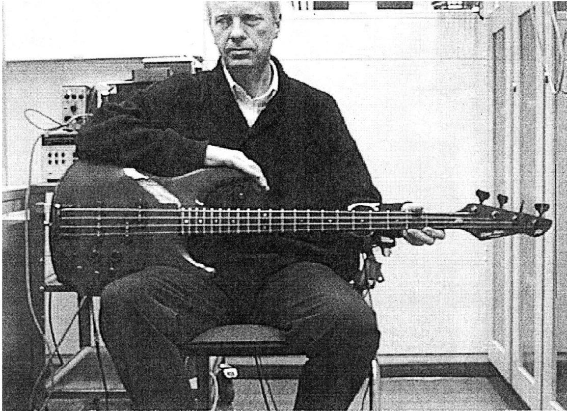
Fig. 22. Dyna Bass No. 3 during the experimental determination of the operating deflection shapes by means of the Scanning Vibrometer.
