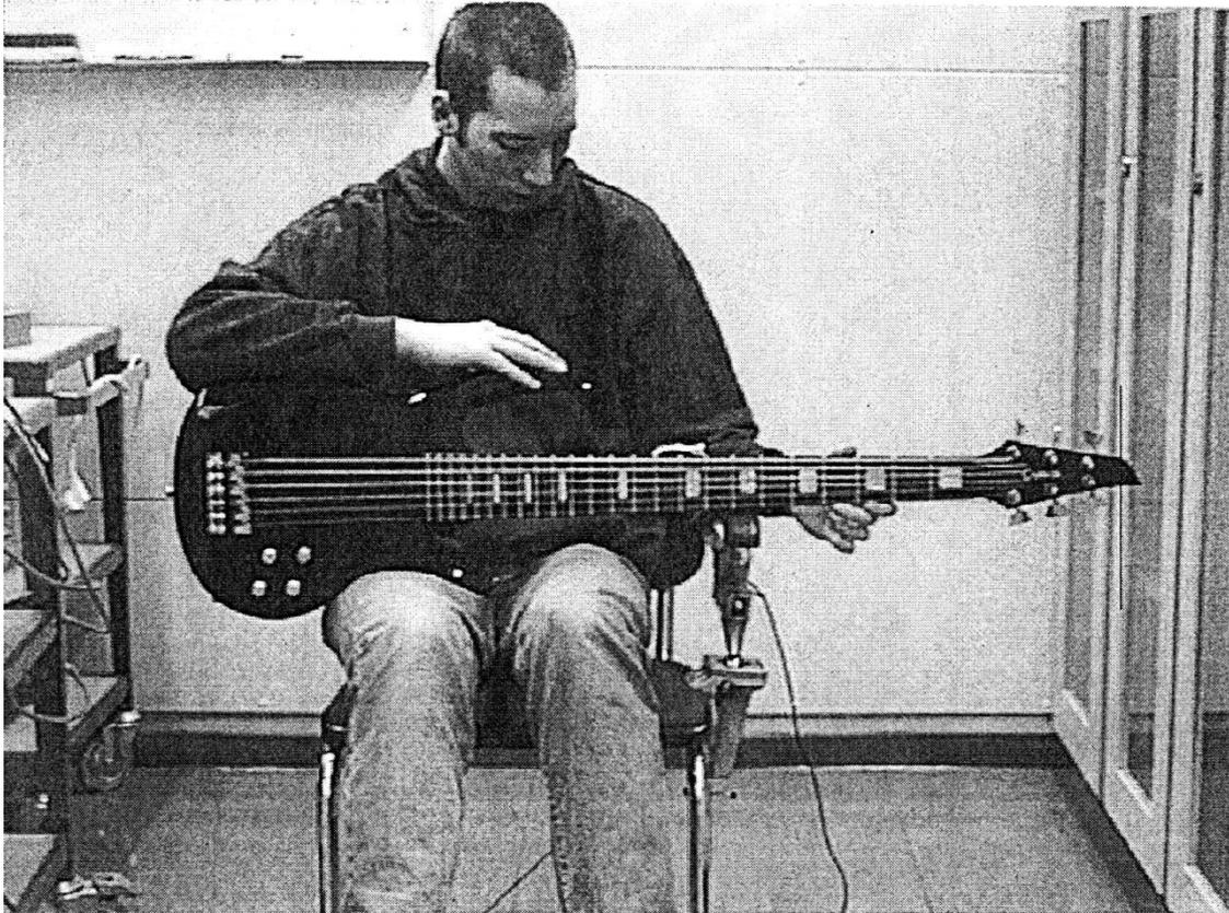
*Fig. 25. Carvin Bass No. 4 during the experimental determination of the operating deflection shapes by means of the Scanning Vibrometer.*
