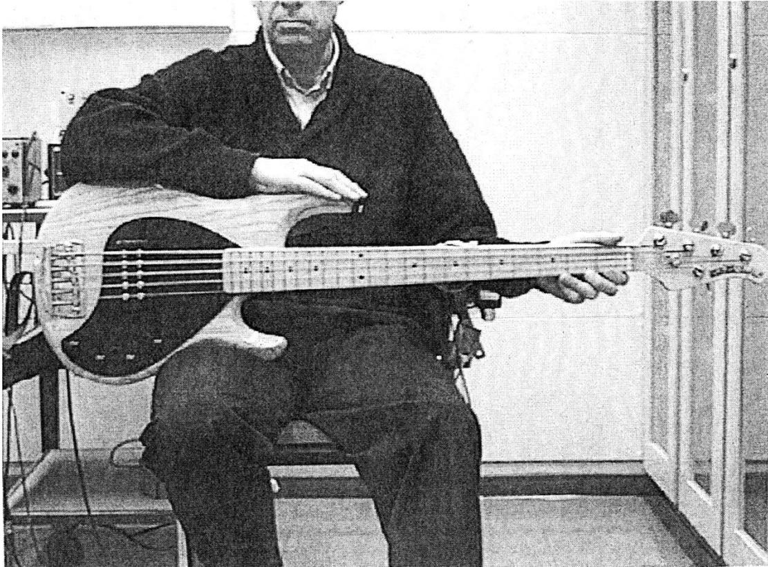
*Fig. 19. Music Man Bass No. 2 during the experimental determination of the operating deflection shapes by means of the Scanning Vibrometer.*
