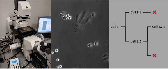
Figure 1:On the left the microscope is shown with a live-cell-imaging set-up installed. In the middle a phase-contrast image of CHO-cells is depicted and on the right an example lineage for cells. Our aim is to create from phase-contrast videos such lineages for every cell and analyze them with CeCILE.
