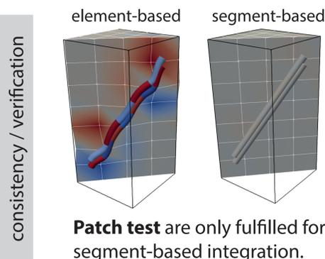
Patch test are only fulfilled for segment-based integration.
