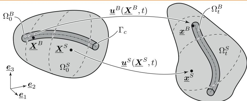
In the beam-to-solid volume mesh tying case the displacements of the beam surface are coupled to the solid, via
