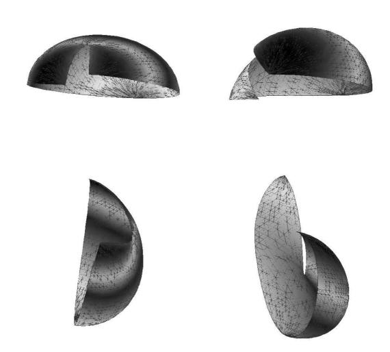
Figure 3: 3D illustration of the eigenfunctions (left: Bazant-Estenssoro crack,  $\xi=45^\circ$ ,  $\alpha=0.684$ ; right: Crack problem  $\xi=45^\circ$ ,  $\alpha=0.388$ ) shown from different viewpoints
