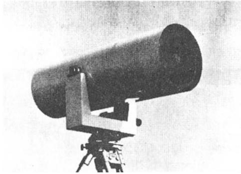
The Terrameter's range varies from 350 m to 15 km. The outgoing power of the He-Ne laser is 5 mw and that of the He-Cd laser is 10 mw. The polarisation is modulated at 3 GHz, i.e. a modulation wavelength of 10 cm. The beam dispersion is limited by the atmosphere at  $2 \cdot 10^{-4}$  radians.
