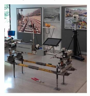
The operator controls the interactive measuring process via a touch screen display. The GML software communicates via an open interface with the parallel running alignment software, which provides the target geometry of the route to be set out. Ordinarily one person is required to operate the measuring system and two persons are required for transport.
