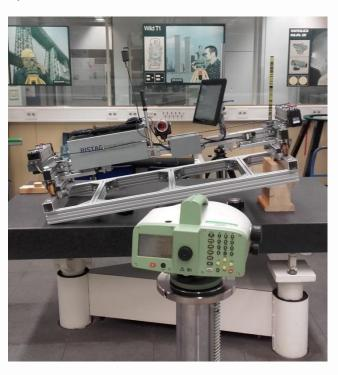
During the project, a system calibration can be carried out on site with the aid of a special frame construction, which was previously referenced with the Leica AT901-LR laser tracker. Special adaptations allow the use of barcode levelling staffs to check the inclination sensor if the frame is tilted.
