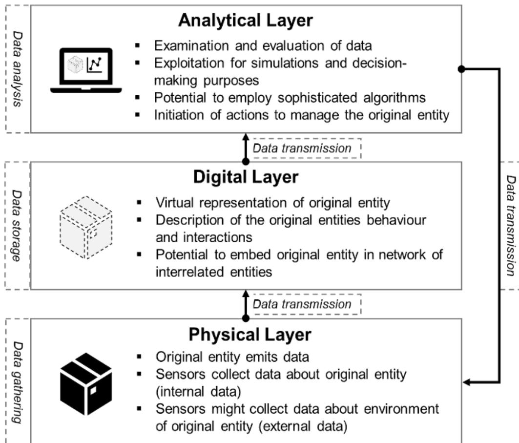
**Figure 5. Basic Digital Twin architecture**
